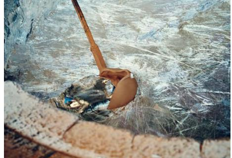
Door-handle blanks are treated for several hours in a vibratory tumbler. This is where they attain the consummate quality so typical of FSB: their radii and edges are painstakingly gone over with a small ceramic sphere.
